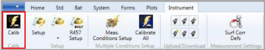
3. Select **Calibration**. The measurement main window displays:
