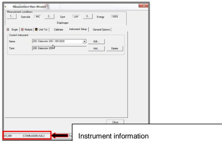
9. Click **Close**. The Measurement Main Window displays. You can now calibrate the instrument.
