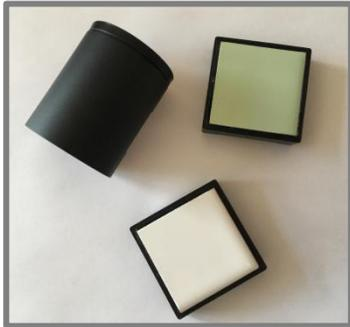
The software prompts for instrument calibration vary slightly from one program to another. However, you are always required to measure the black trap, white tile and green tile to complete the calibration.
