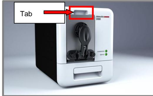
2. Pull the tab down to its full horizontal position. Look at the backside of the door to see the area of the port opening that is covered by the sample.
