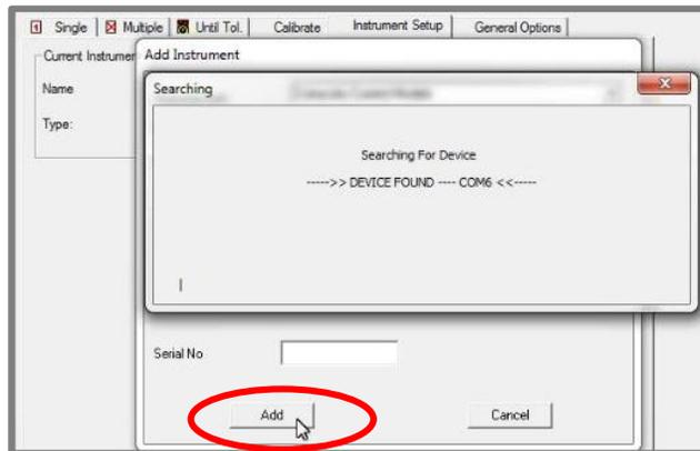
8. Click **Add**. Datalogic 200 will display as the current instrument. At the bottom of the window, the program will display information about the instrument selected:
