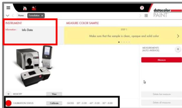
2. The program will locate the instrument and the screen will display information about the instrument that is connected. The *Calibration Status* will be **red**.
