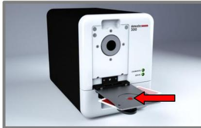
If necessary, adjust the placement of the sample to properly position the sample area to be measured. The sample must completely cover the port opening.
