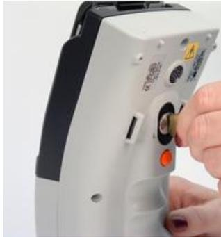
4. Calibrate the instrument. Following calibration, the aperture icon on the PDA screen should match the switch position on the back of the unit, and the aperture identification on the stapler foot assembly.
