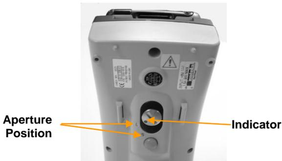
3. Turn the switch to the position that matches the stapler foot aperture size.
