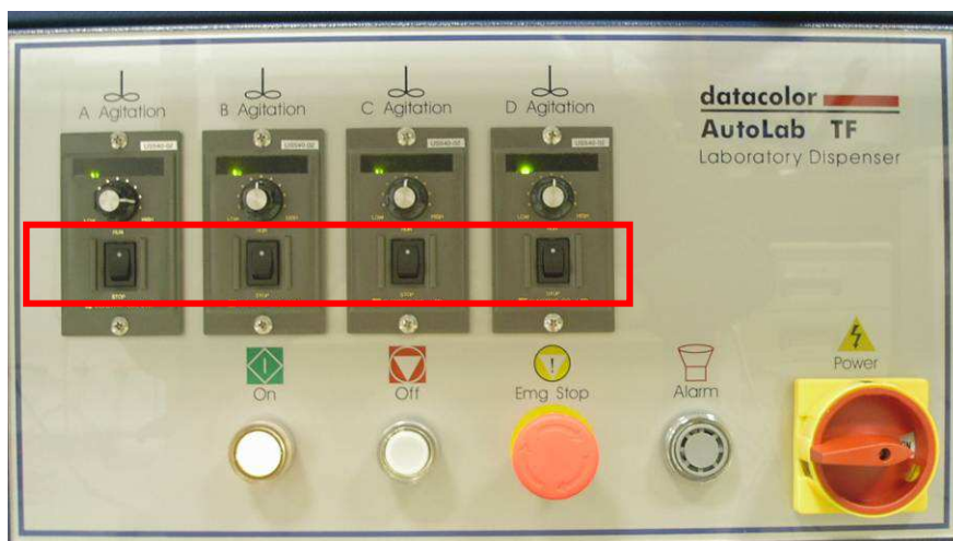
Step 3: Ensure that all agitation controller switches are in the “ON” position
