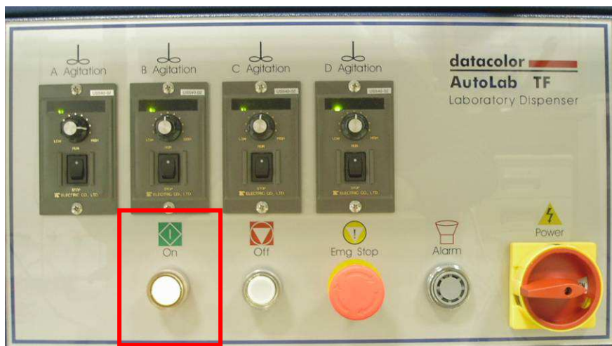
Step 2: Press the “ON” button to power up the system. The “ON” button will illuminate
