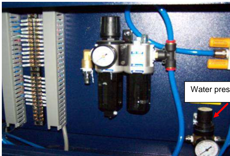
Step 5: Check to ensure the water pressure is between 0.8~1 kg/cm 2 .
